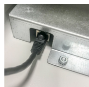
RJ45 cable connected to keypad on underside of front panel. Release cable before removing cover.
